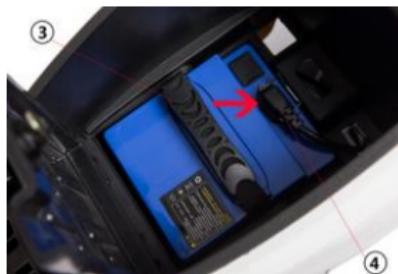
① Open the cap of battery case with the key,plug the battery cable inside the socket,connecting the battery with scooter.
