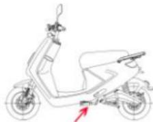
③ Insert the key and turn rightwards, "Powered" state is started, the Instrument is opened, and the "READY" light is ON, scooter is ready for driving.
